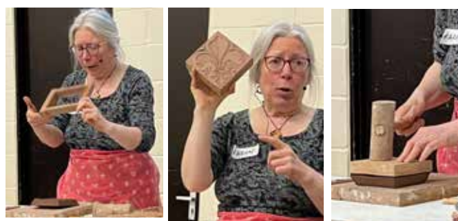
The tile is banged out of the mould and a carved wooden block impressed onto the surface.
