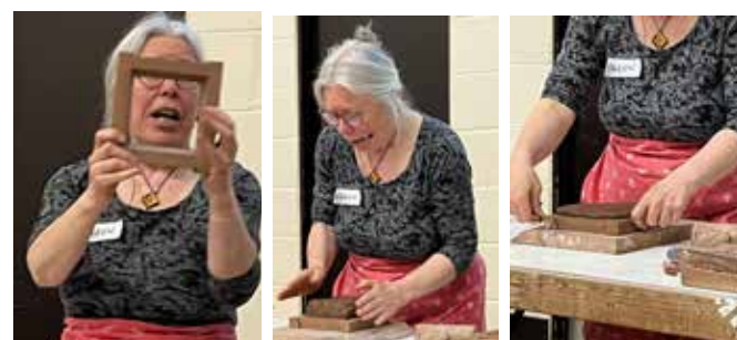
Karen presses the clay into the square mould then wires off the top to create a flat surface, which can then be smoothed.
