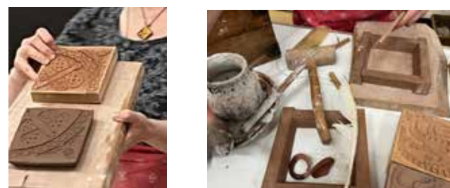
A wooden block and a tile impressed from it. Tools of the trade: moulds, a mallet and carved wooden blocks.
