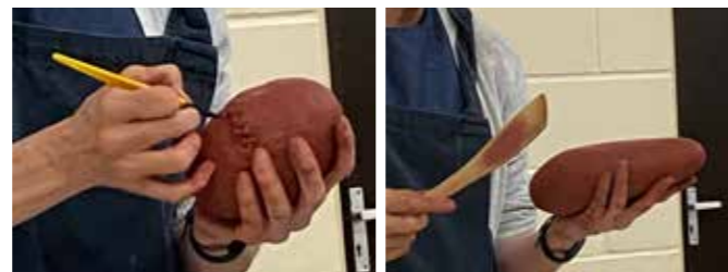
Joining two pinch pots and paddling the form to elongate the shape.
