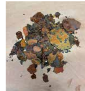
Flakes of iron rust from an old gas kiln used in glazes and clay bodies.
