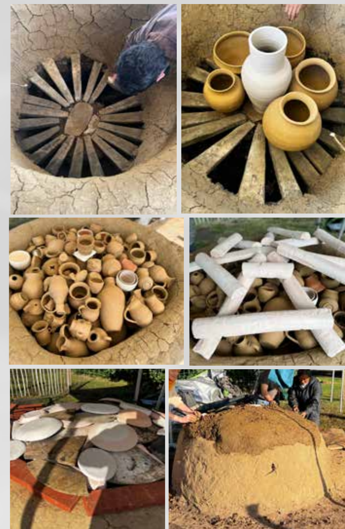
Above: Loading and sealing the kiln. Left: First glimpse of the fired pots. Far Left: "Mooki" in mid-fire. Below: Blackened, almost metallic, heavily reduced pots. There were casualties with cracks and distortions, but many pots survived intact.
