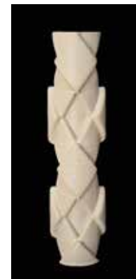
Very precise, geometric designs can be achieved with 3D printing, and porcelain lends itself to the printing process, being smooth and fine to work with.
