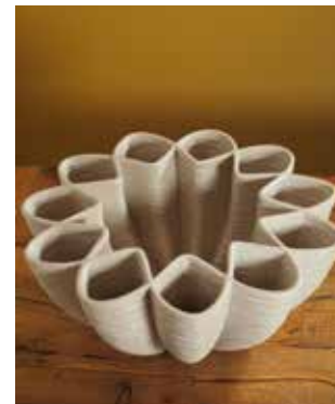
Very precise, geometric designs can be achieved with 3D printing, and porcelain lends itself to the printing process, being smooth and fine to work with.
