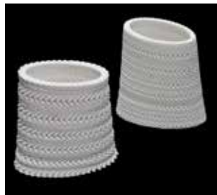
An intricate design taking advantage of the fact the technology prints using tiny coils allowing for fine detail and the creation of some stunning pots.
