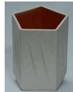
Very precise, geometric designs can be achieved with 3D printing, and porcelain lends itself to the printing process, being smooth and fine to work with.
