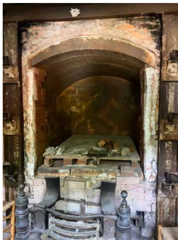
Above: Enormous diesel-fired trolley kiln.
