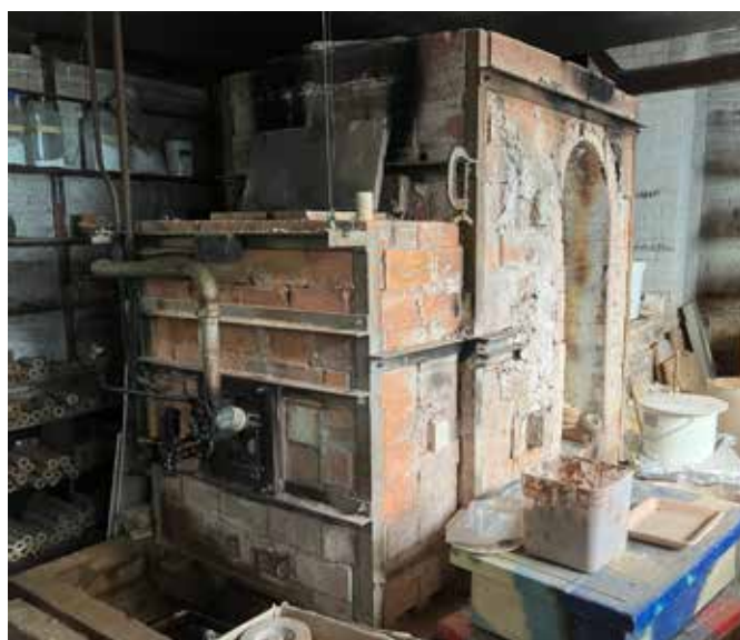
Above: Enormous diesel-fired trolley kiln.
