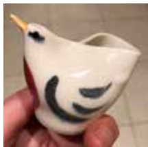
Underglaze running, bloating and crazing – TRIPLE whammy.
