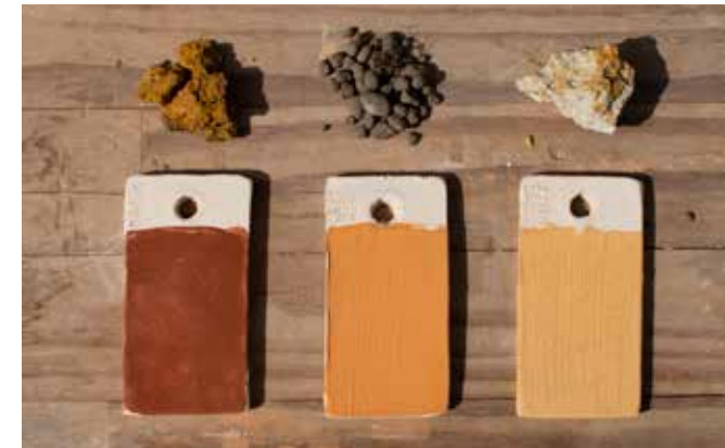
Wild slip test tiles with their source clays
