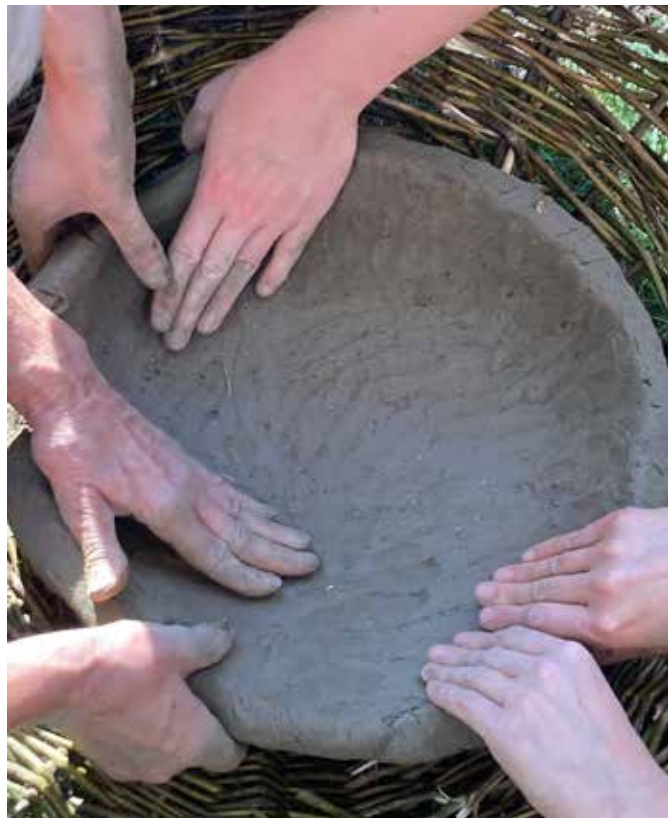
Making the clay dome roof for the kiln
