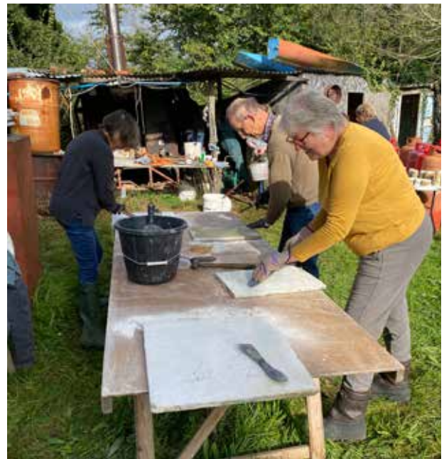
Cleaning and batwashing the kiln shelves
