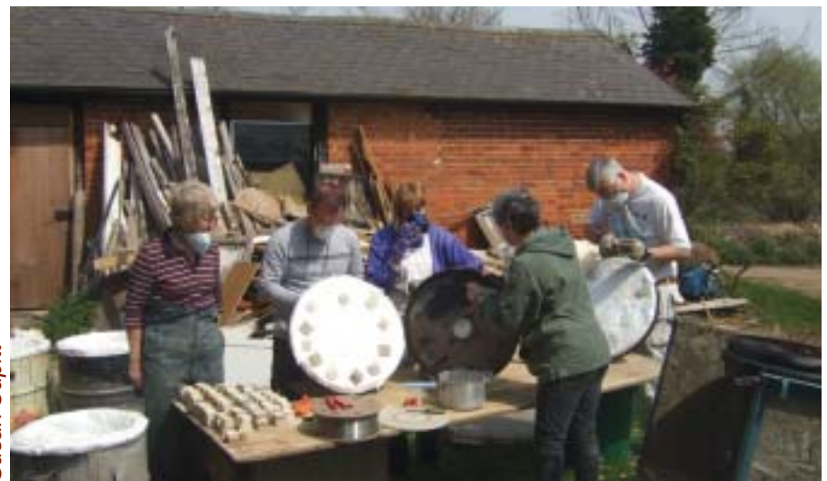
Raku Kiln Building weekend, fitting buttons to lids
